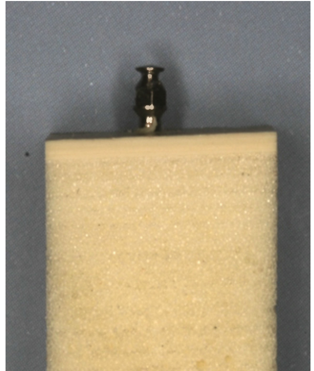
Figure 2. Photograph of an MI inserted in synthetic bone block with 1-mm-thick cortical bone layer.
