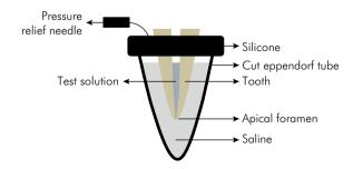
**Figure 1.** Schematic of the test system. The sample was attached to an Eppendorf tube using an individual silicone plug. A disposable 27-G needle was inserted into the silicone plug to balance the internal and external pressures. The Eppendorf tube was filled with 0.8 mL of sterile saline solution. The root canal was filled with 0.02 mL of the test solution.
