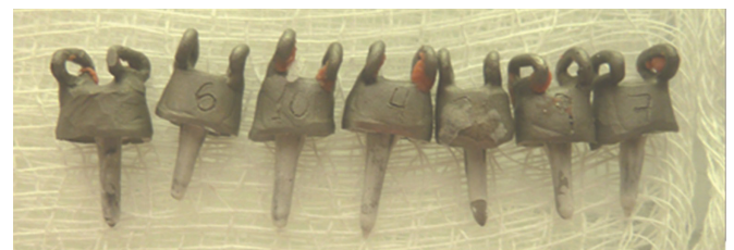
Figure 1. Cast metal post-core assemblies and copings separated as a whole after being subjected to tensile stress.
