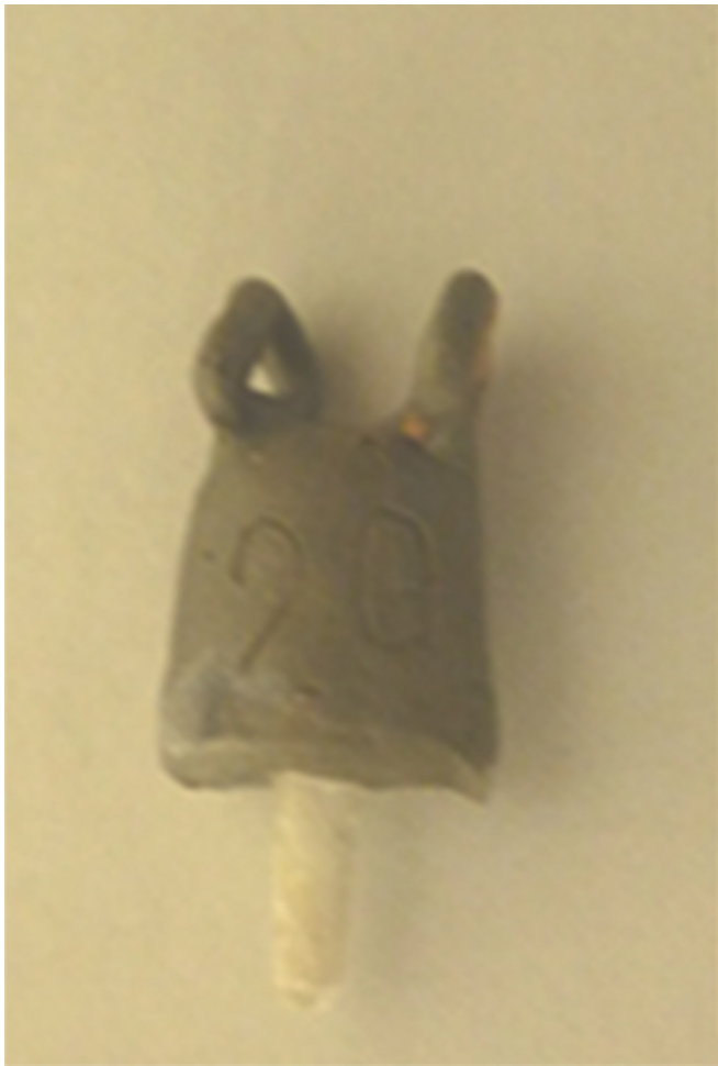
Figure 2. Glass-fiber post-core assembly and coping separated as a whole after tensile testing.
