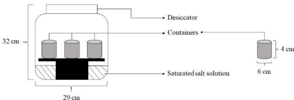
**Figure 1.** Schematic drawing of the samples and saturated salt solutions inside the hermetic desiccators used in the experiment.
