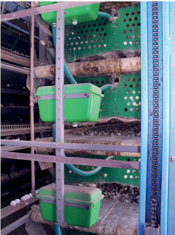
**Figure 2.** Poultry houses with manure removal through mechanical treadmills.
