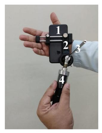
**Fig. 1** Set of equipment consisting of 1) a smartphone; 2) an adaptor; 3) a telescope and 4) a light source.
