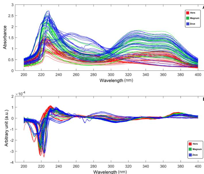
**Figure 1.** Original (A) and pre-treated (B) data of the three types of hops studied, in all storage conditions (a, b, c and d) and storage times (0, 1, 2 and 3), by UV-Vis spectrophotometry between 200 and 400 nm. Samples of *Hersbrucker* (—), *Magnum* (—) and *Zeus* (—) hops.
