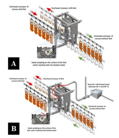
Figure 1. Schematic designs of the operational self-washing system of the feet-cutter disc with (A) non-heated and (B) heated water.
