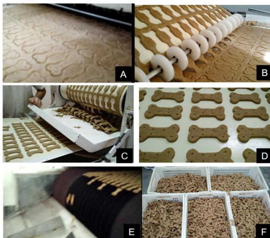
**Figure 1.** Pet biscuit production line. (A) Cutting the biscuits. (B) Separation of the cut biscuits from the dough cylinder, passing through the conveyor belt. (C) Biscuits on the baking mat and the residue returning to be rolled again. (D) Cut biscuits passing through the conveyor belt. (E) Baked biscuits coming out of the oven. (F) Ready-made biscuits.
