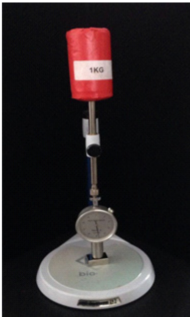
Figure 2. Device used to perform the Shore A hardness evaluation.
