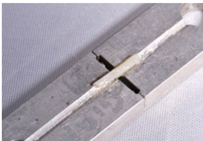
Figure 2. The specimen attached to the microtensile device.
