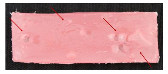
Figure 1. Defects and Pores in the thermoplastic resin specimens.
