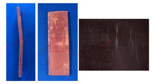
Figure 3. A) Bar specimens of the RTP group after the flexural strength test, the arrow shows the permanent change of the specimen; B) Arrow points area where the chisel was positioned; C) Stereomicroscope image (13x magnification) shows the stress area (arrow) suffered by the specimens during the mechanical test.
