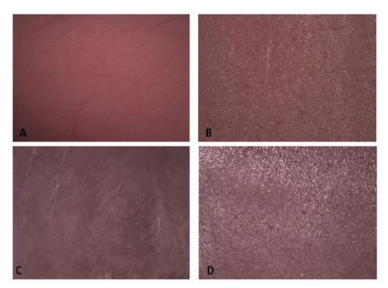
Figure 2. Polished and unpolished surface of the resins under study, A-RAT polished (15x magnification stereomicroscope image), B-RAT unpolished (15x magnification stereomicroscope image), C-RTP polished (12x magnification stereomicroscope image), D-RTP unpolished (12x magnification stereomicroscope image).
