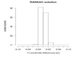
Figure 10 presents the histogram of the Y coordinate differences obtained in the second scenario. The values of these differences are between -0.04 to 0.04 m but more than 90% of the differences are less than  $\pm$  0.02m.
