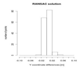
Figure 14 shows the histogram of the Y coordinate differences obtained in the third scenario. The differences are similar to the Y coordinate differences in the second scenario and are between -0.04 and 0.06 m.
