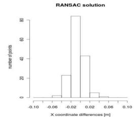
In the Figure 13, the histogram of the X coordinate differences obtained in the third scenario is presented. The values of these differences are between -0.06 and 0.06 m as in the second scenario. The results of the transformation are almost the same in those two scenarios.
