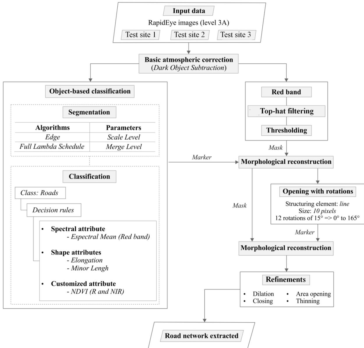
Figure 2: Flowchart of road network extraction methodology.
