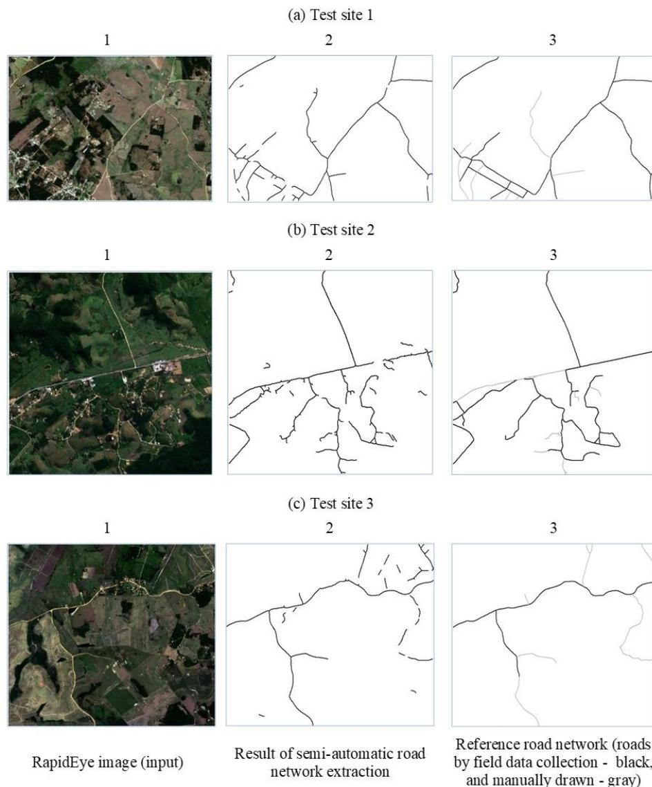
**Figure 4:** Original RapidEye images (a1, b1, c1), semi-automatic extracted road network (a2, b2, c2) and reference road network (a3, b3, c3) used to evaluate the extraction method, for (a) test site 1, (b) test site 2, and (c) test site 3.
