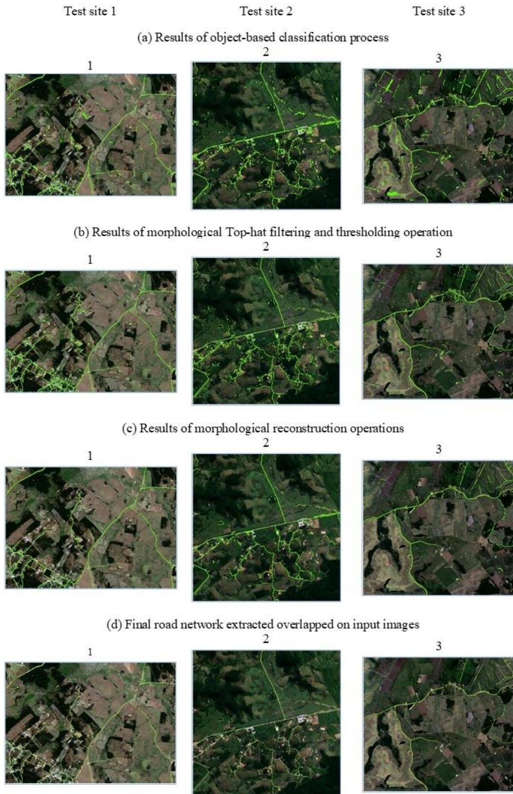
**Figure 3:** Results from main performed steps of proposed methodology for all three test sites (1, 2 and 3). (a) the resultant object-based classification, (b) results of morphological Top-hat filtering and thresholding operation (c) results of morphological reconstruction operations and (d) final extracted road network overlapped on original images.
