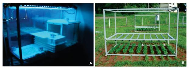
FIGURE 6 - A. Laboratory and B. field facilities to study the effects of increased UV-B radiation on plant diseases and biological control agents (Jaguariúna SP, Brazil).
