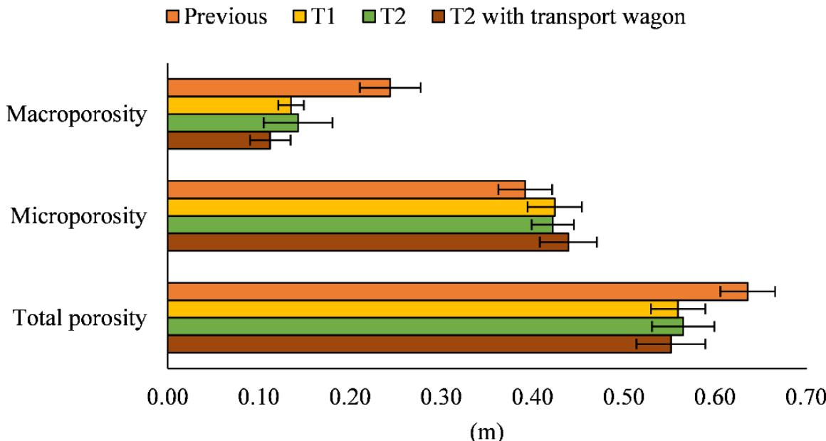
**Figure 2.** Macro, micro, and total porosity (m<sup>3</sup> m<sup>-3</sup>) at the experimental area in the treatments: previous (before silage harvest), T1, T2, and T2 with transport wagon in the layer of 0.0 – 0.2 m.
