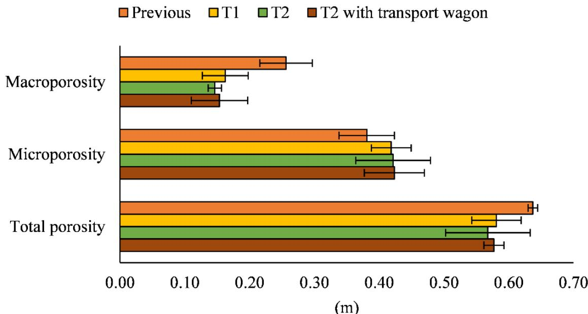
**Figure 3.** Macro, micro, and total porosity ( $\text{m}^3 \text{ m}^{-3}$ ) of the experimental area in the treatments: previous (before silage harvest), T1, T2, and T2 with transport wagon in the layer of 0.2 – 0.4 m.
