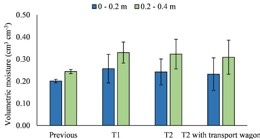
**Figure 4.** Volumetric soil water content ( $\text{cm}^3 \text{cm}^{-3}$ ) of the experimental area in the treatments: previous (before silage harvest), T1, T2, and T2 with transport wagon in the evaluated layers.
