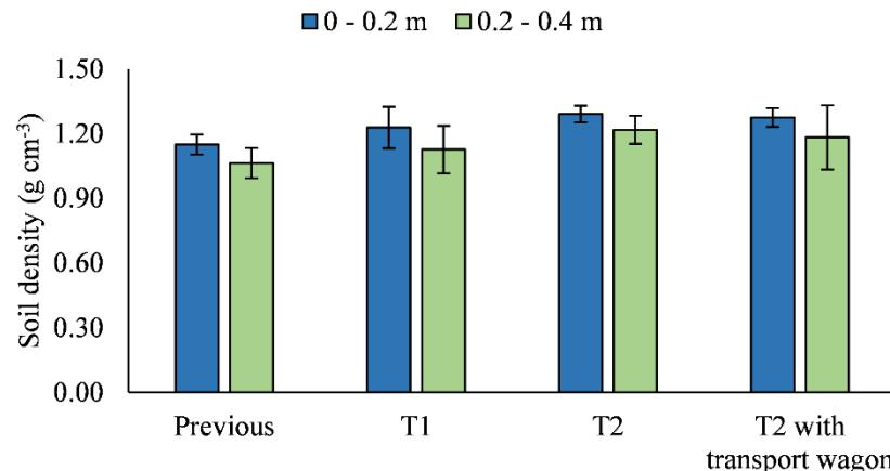
**Figure 5.** Soil density ( $\text{g cm}^{-3}$ ) of the experimental area in the treatments: previous (before silage harvest), T1, T2, and T2 with transport wagon at the evaluated depths.
