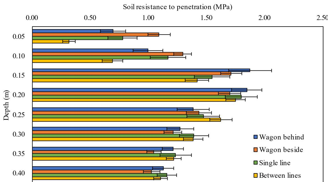
**Figure 6.** Resistance to soil penetration (MPa) of the experimental area in the treatments: T1, T2, and T2 with transport wagon.
