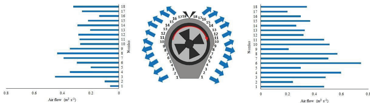
Figure 1. Distribution profile of airflow from the hydraulic nozzles of both sides of an axial fan sprayer.
