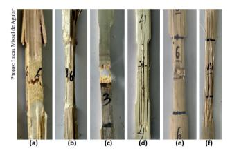
Figure 3. Fractures observed in the tested specimens from culms of *Dendrocalamus asper* with (a) and without node (b), *Phyllostachys pubescens* with (c) and without node (d), and *Phyllostachys aurea* with (e) and without node (d).
