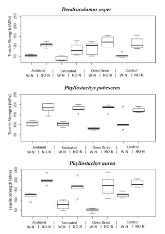
Figure 4. Dispersion of the tensile strength parallel to the fibers for the tested specimens. W-N: with node; NO-N: without node.
