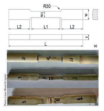
Figure 2. Representation of the tested specimens and their dimensions (a; W=width; L=length; t=wall thickness; R30 = radius of 30 mm), with *Dendrocalamus asper*, *Phyllostachys pubescens* and *Phyllostachys aurea* from the bottom to the top (b).
