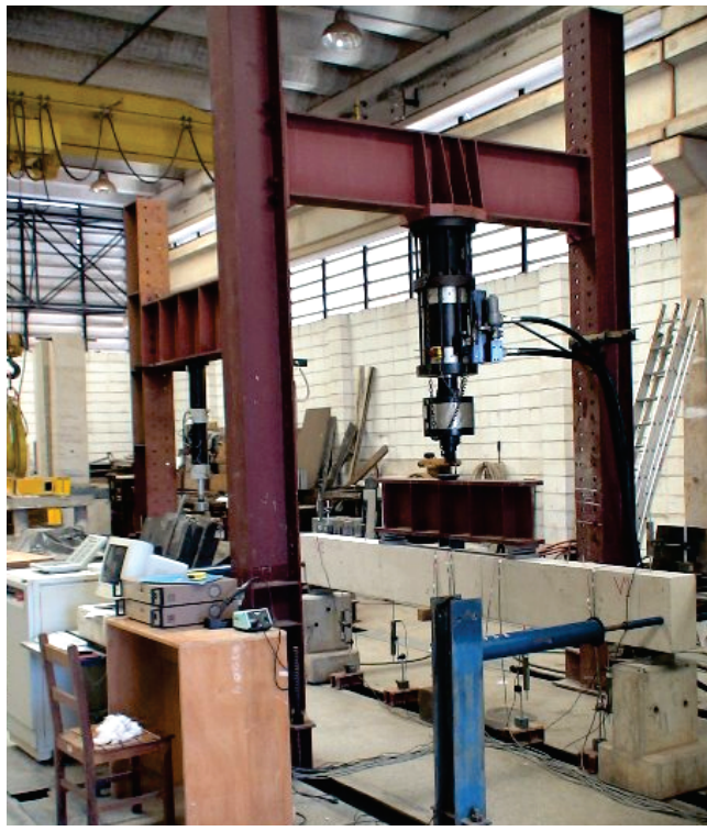
Figure 9 – Schematic of the flexural test of beams
