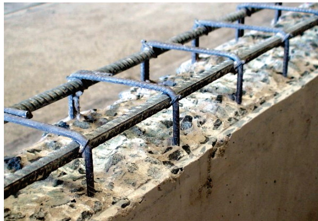
Figure 7 - Removal of concrete from the tensile zone of the beam V2C
