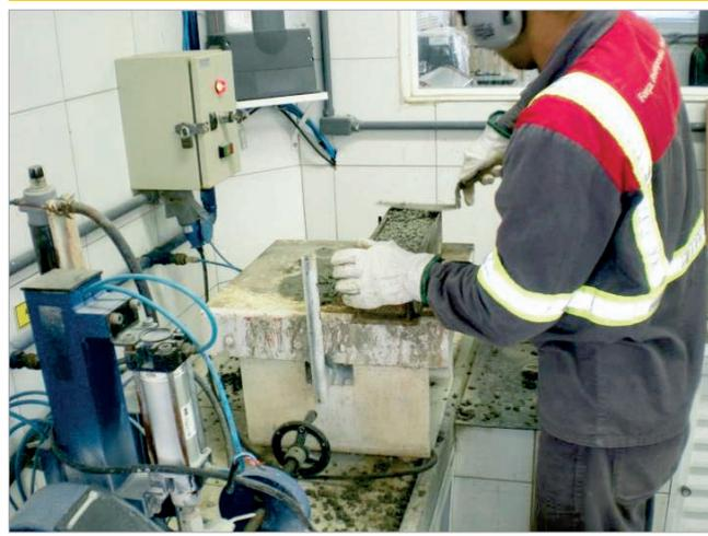
During the test the samples were wrapped in plastic film in order to avoid loss of water through its lateral surface. Furthermore, two silicone rings were used for sealing the bottom and the top of the samples were produced, avoiding water leaks during the tests. The tests were carried out 25 days after molding.
