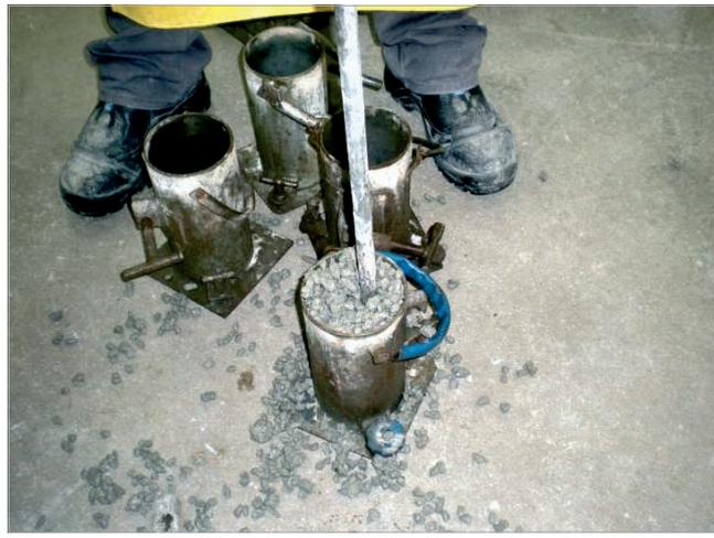
stable structure to be demolded after 24 hours, as recommended by the Brazilian standard.
