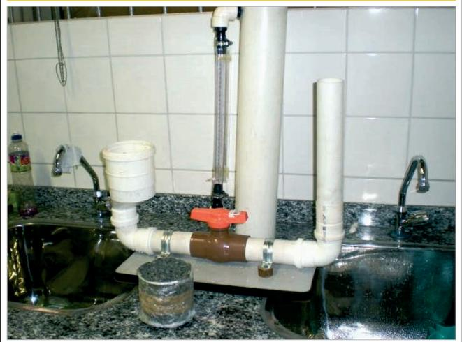
Figure 4 – Constant head permeameter
