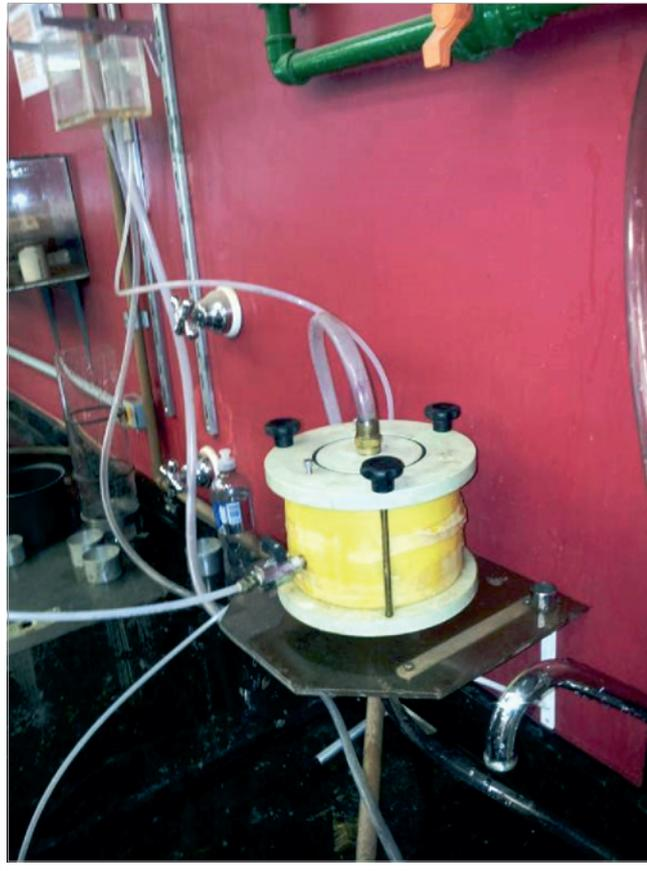
The apparatus is equipped in the bottom with a plastic ring where the specimen is placed (Figure 4). A flexible membrane positioned internally on the plastic ring is pressurized on the side of the samples in order to avoid water leaks by its lateral during the test. The container used to produce the water pressure is provided with an inlet and an outlet of water as well as by a lower safety outlet to prevent overflow.
