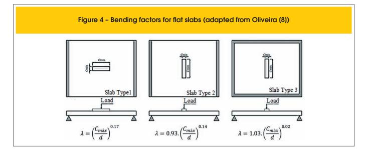
a value of the flexural factor ( $\lambda$ ) was proposed for the correction of the theoretical punching resistance, as shown in Figure 4.
