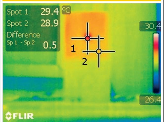
Figure 22 - CP3, group 1, EPS  $\phi=6$  cm, heated by high-pressure sodium lamp
