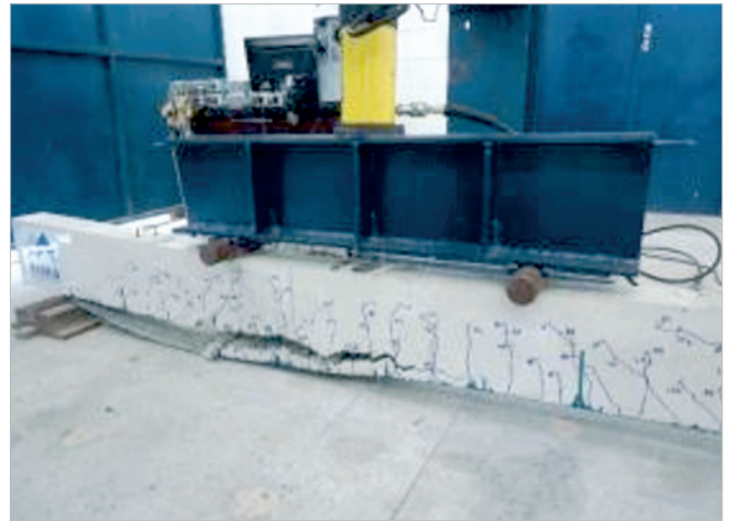
B VA-2 beam in the collapse
