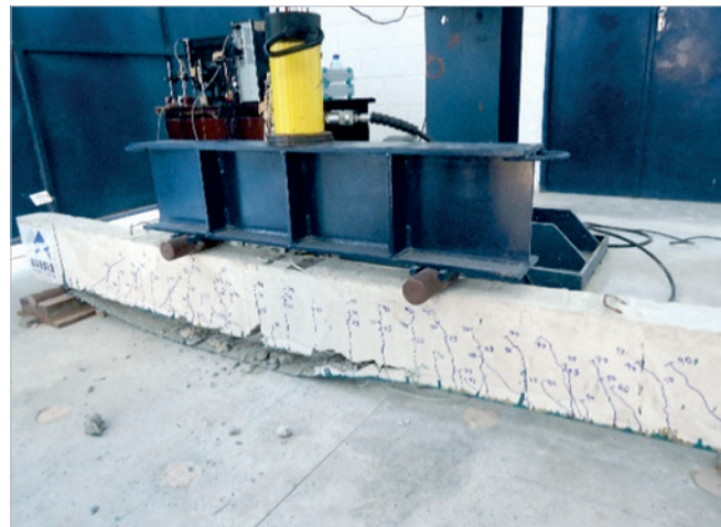
B VB-2 beam in the collapse
