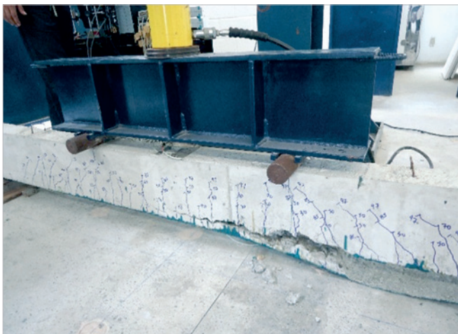
C VB-3 beam in the collapse
