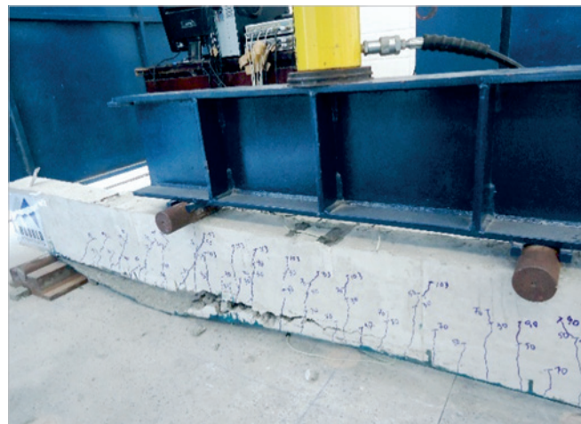
D VB-4 beam in the collapse
