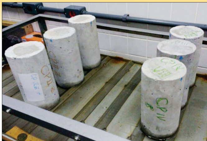
Figure 4 Capillary absorption test of specimens (procedure of NBR 9779 [27])
