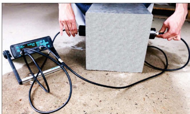
Figure 5 Transducers positioning mode for ultrasonic pulse emission and reception in 25 cm cubic edge specimens
