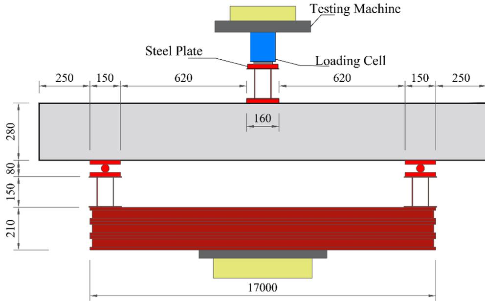
Figure 3. Testing setup
