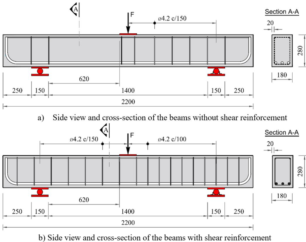
**Figure 2.** Flexural and shear reinforcement of the tested beams
