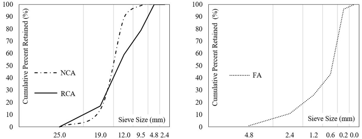
a) The granulometric curve of coarse aggregate      b) The granulometric curve of fine aggregate
