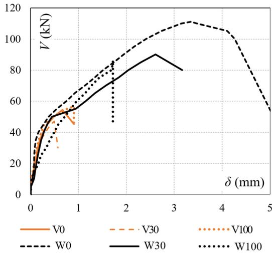
**Figure 6** –  $V - \delta$  response of the tested beams.
