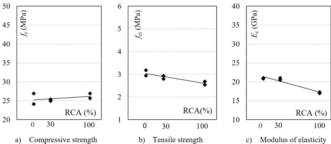
Figure 5 – Results of characterization tests.
