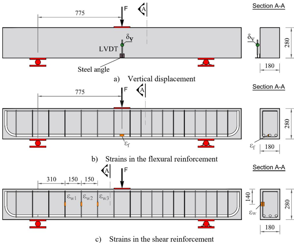
Figure 4. Instrumentation of the tested beams.
