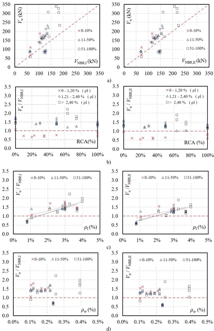
Figure 8. Comparison between the experimental and theoretical for the database of beams with stirrups
