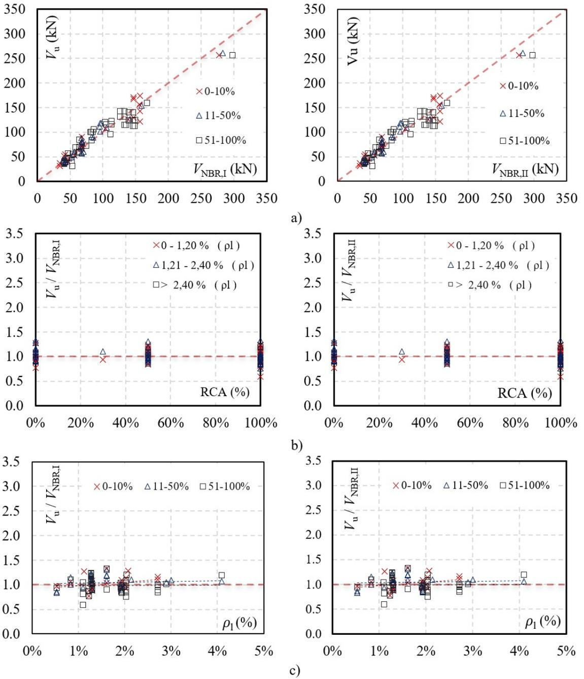
Figure 9. Comparison between the experimental and theoretical for the database of beams without stirrups
