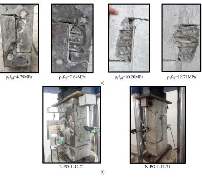
Figure 8. Modes of shear failure of push-off specimens: a) shear plane failure, b) bending and shear combination failure [15].
