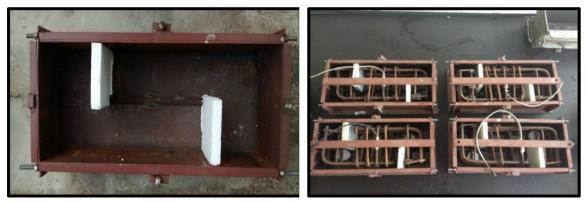
Figure 4. Metallic form for the production of push-off specimens [15].
