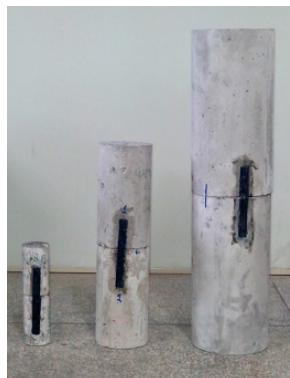
**Figure 6.** Variation in specimen dimensions.**Table 2.** Experimental program.
