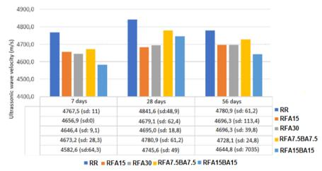
Figure 6 – Ultrasonic pulse velocity test results
