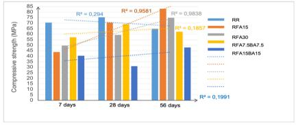
Figure 5 – Compressive strength test results
