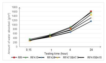
Figure 7 – 28-day capillary water absorption test results
