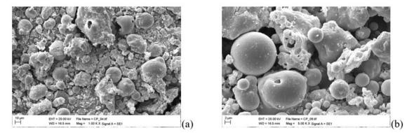
Figure 4 – Shape of the coal bottom ash used in this study, assessed by scanning electron microscopy
