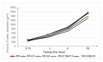
Figure 8 – 56-day capillary water absorption test results
