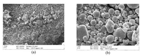
Figure 3 – Shape of the fly ash used in this study, assessed by scanning electron microscopy
