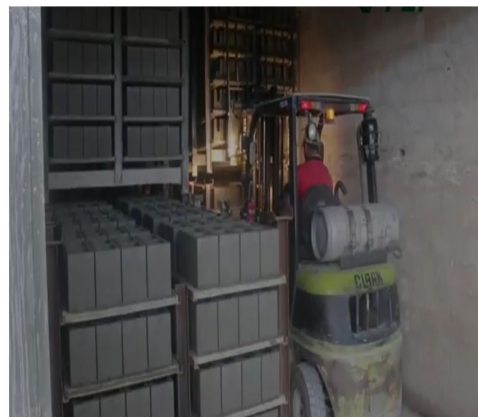
Figure 15. Steam curing chamber in a concrete block industry in the state of São Paulo. Source: Author (2022).
