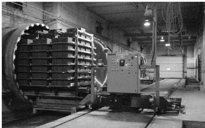
Figure 7. Carbonation chamber developed by Carboclave. Source: [[35]].
