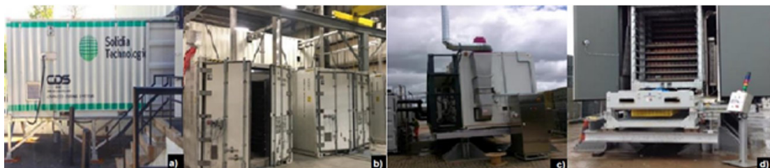
Figure 4. Carbonation chambers developed in Container structures, located: a) USA, b) Canada, c) d) UK. Source: [33].
