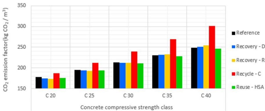
Figure 4. CO<sub>2</sub> emission of 1 m<sup>3</sup> of concrete with 100 mm slump, for different concrete types.
