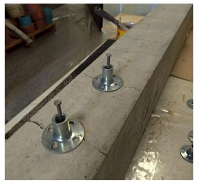
Figure 4. Surface packers secured with nails.
