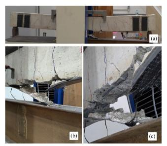
Figure 18. Failure of beam CR63-NI (a); Detail of the rupture and debonding of the CFRP sheet (b); Detail of the non-rupture of the positive reinforcement (c).
