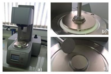
Figure 4. a) rheometer; b) addition of the paste c) geometry - cross hatched.
