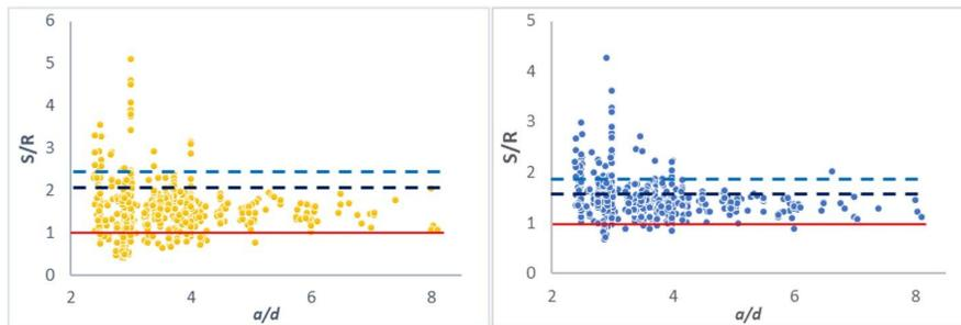
Figure 5 - S/R in relation to  $a/d$  to ACI 318 [3] (yellow) and ACI 318 [3] (blue)
