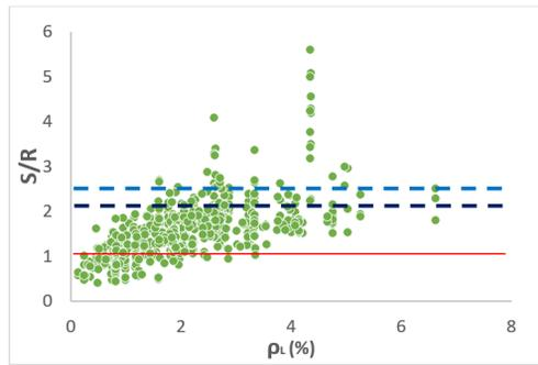
Figure 14- S/R in relation to  $\rho_L$  to NBR 6118:2014
