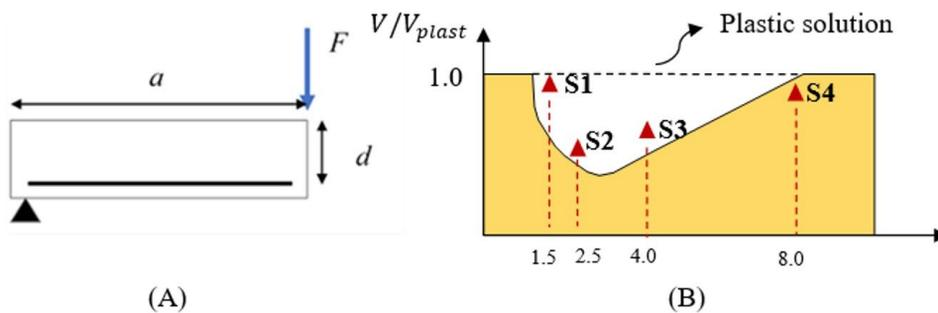
Figure 1 – (A) Shear span ( $a$ ) to effective depth ( $d$ ) to a point load (B) Kani's valley
