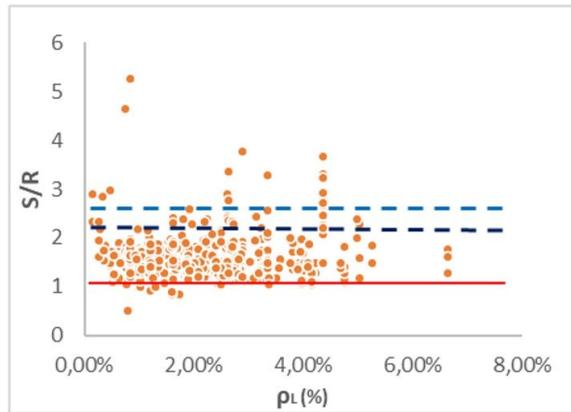
Figure 10- S/R in relation to ρL to Frosch et al. [5]
