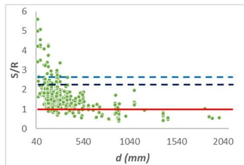
Figure 15- S/R in relation to  $d$  to NBR 6118:2014
