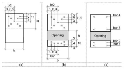
Figure 4 – Temperature reading points in the cross-section of the beams (a) without and (b) (c) with openings
