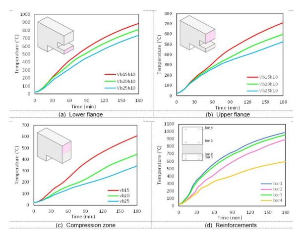
Figure 5 – Thermal field in (a) lower and (b) upper flange of the concrete (beam with opening), (c) in the compresses region of the concrete (beam without opening) and (d) in the reinforcements
