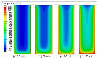
Figure 7 - Thermal field for different ISO 834 times (beam without opening)
