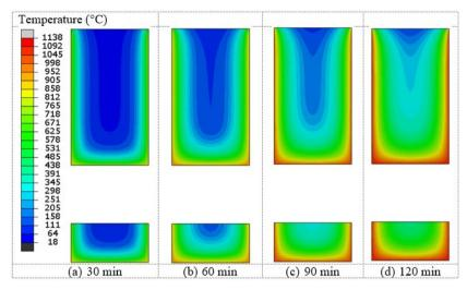
Figure 8 – Thermal field for different ISO 834 times (beam with opening)
