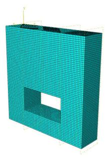
Figure 2 - Computational thermal model (beam with opening)
