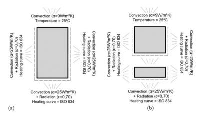
Figure 3 - Heating surfaces in the cross-section of the beams (a) without and (b) with opening
