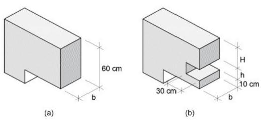
Figure 1 – Beams cross-section (a) without and (b) with openings
