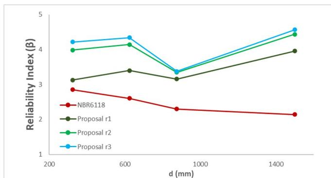
**Figure 6 –** Reliability indexes ( $\beta$ ) in relation to  $d$  to NBR6118:2014 and proposal: C20
