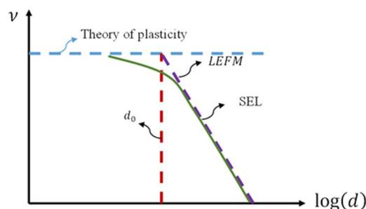
**Figure 1** – SEL asymptotic approach: nominal shear strength ( $v$ ) in terms of cross-section depth  $d$  (log scale).
