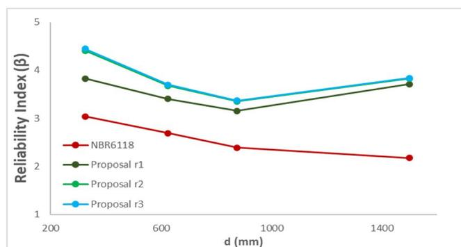
Figure 9 – Reliability indexes ( $\beta$ ) in relation to  $d$  to NBR6118:2014 and proposal: C30
