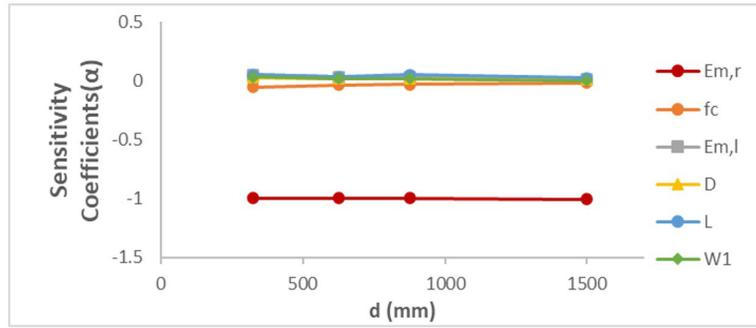
Figure 10 – Sensitivity coefficients to NB6118:2014 to C30
