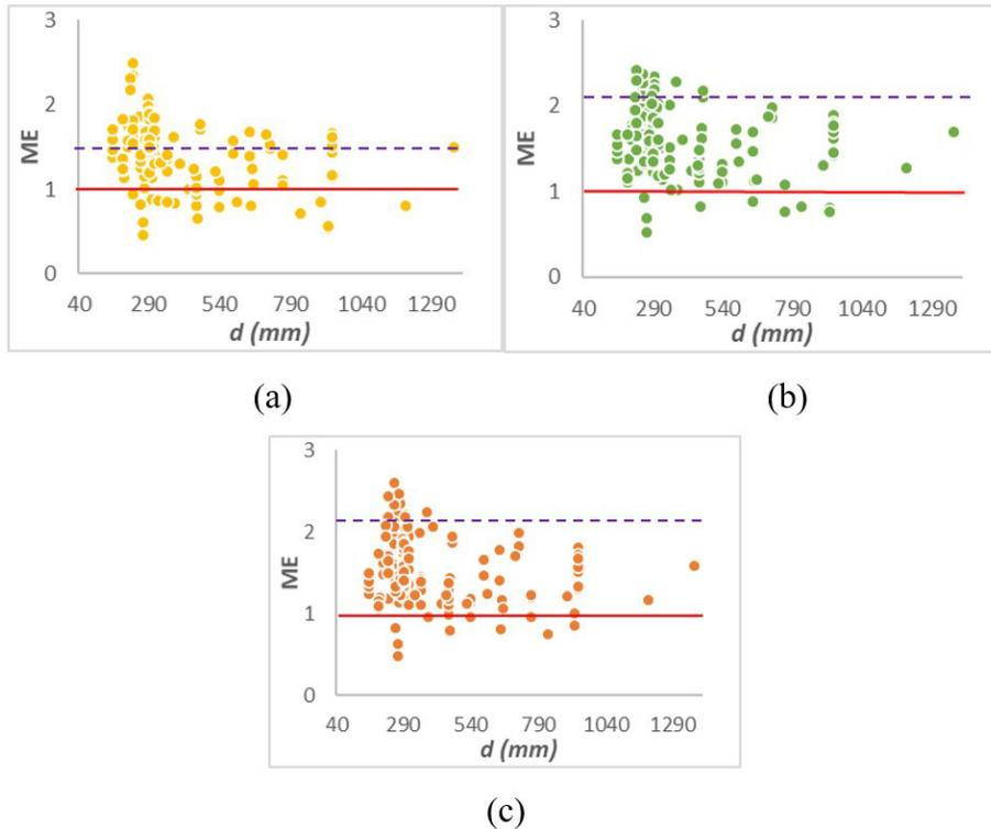
**Figure 16** – ME x  $d(mm)$  for beams with transversal reinforcement: ACI 318: 2019 (a), NBR 6118-14 (b), and Frosch et al. [27] (c)
