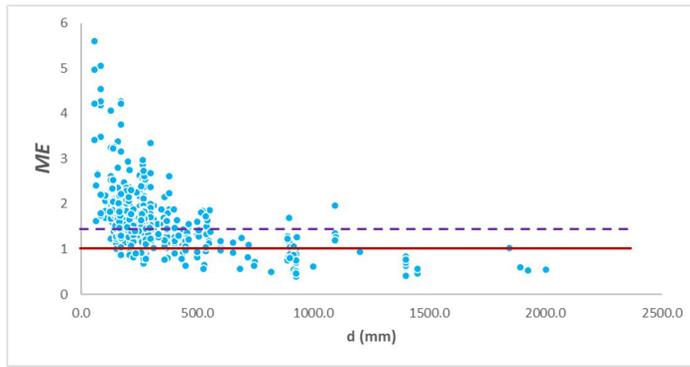
**Figure 4** – ME in terms of  $d$  after application of  $\rho_L$  factor
