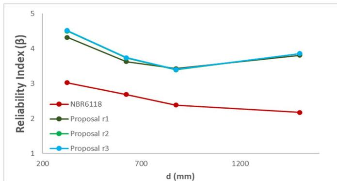
Figure 12 – Reliability indexes ( $\beta$ ) in relation to  $d$  to NBR6118:2014 and proposal: C40
