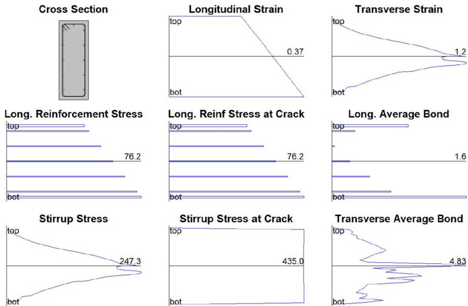
Figure 19. Results related to the reinforcement – Response-2000
