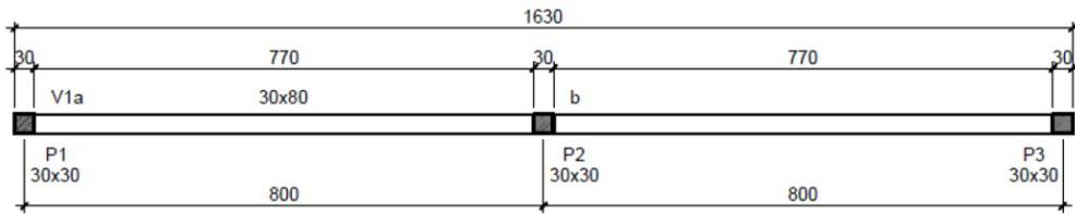
Figure 13. Formwork drawing of the analyzed beam
