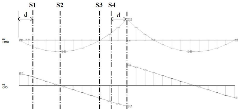
Figure 15. Diagrams of bending moments and shear forces and selected sections.
