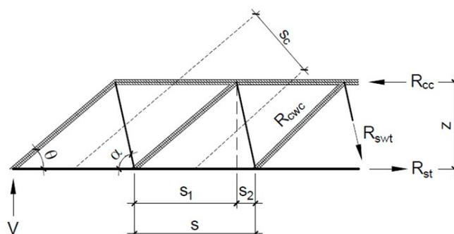
Figure 1. Generalized concrete strut
