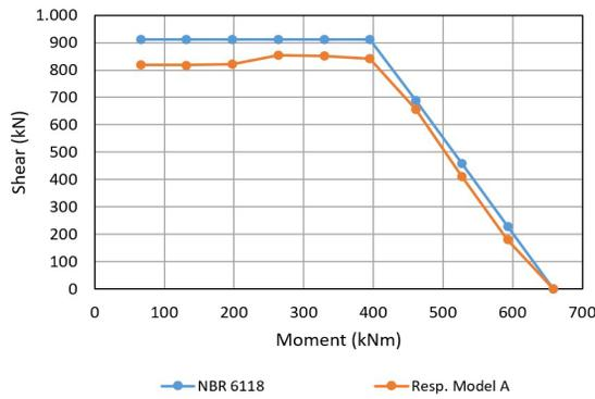
Figure 8. Shear forces obtained with  $\theta_1$ . symmetrical reinforcement
