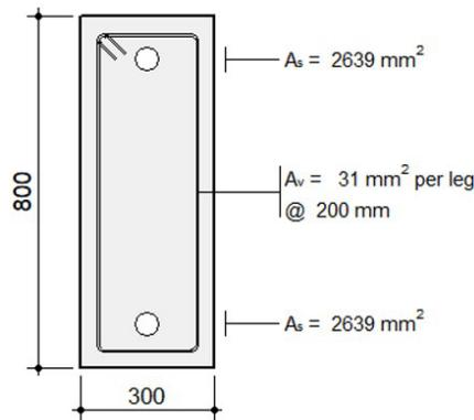
Figure 7. Transversal section with symmetrical reinforcement
