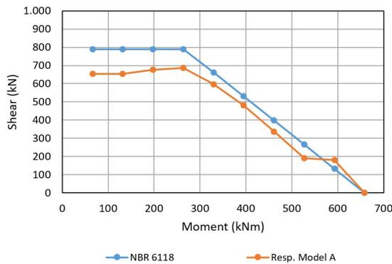
Figure 9. Shear forces obtained with  $\theta_2$ . symmetrical reinforcement
