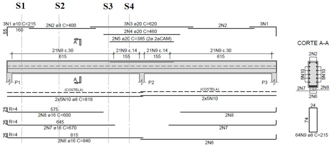
**Figure 16.** Reinforcement detailing
