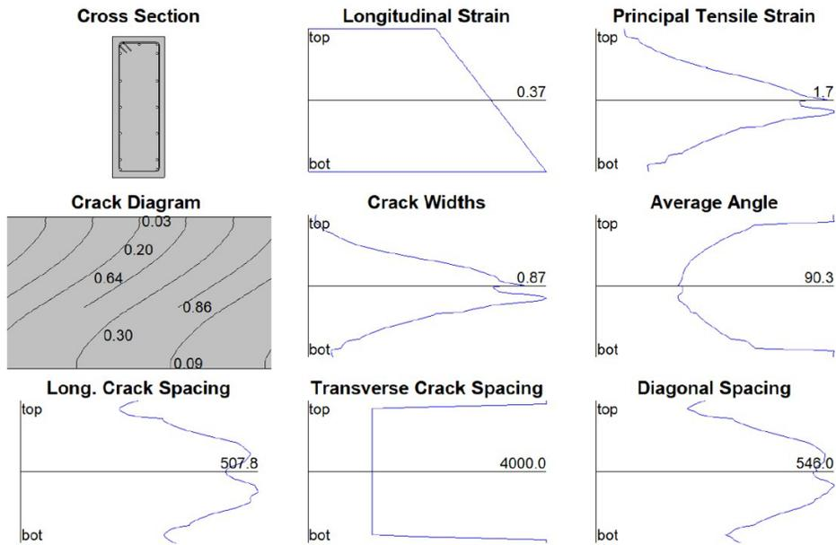
Figure 18. Results related to the cracks – Response-2000
