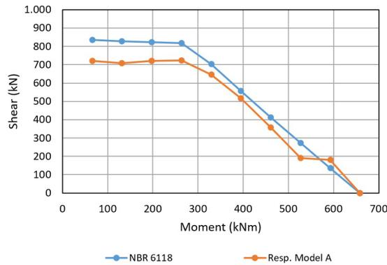
Figure 10. Shear forces obtained with  $\theta_3$ , symmetrical reinforcement
