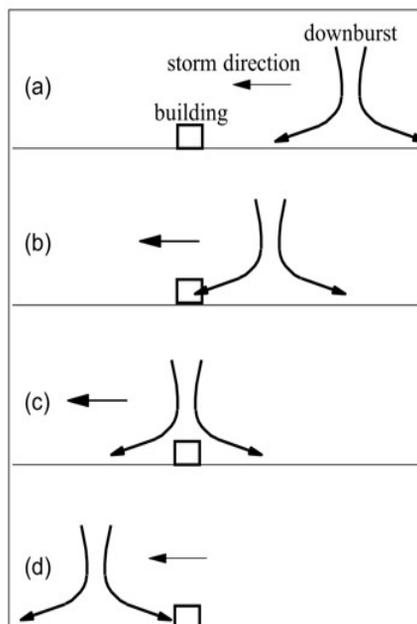
**Figure 6.** Schematic illustration of the passage of a non-stationary downburst by a building (based on Chay et al. [24]).
