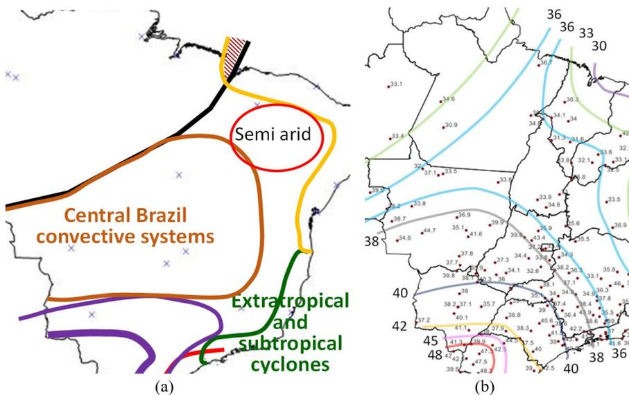
Figure 21. Center and southeast region: a) climatic regions; b) proposed isopleths ( $V_0$  in m/s).
