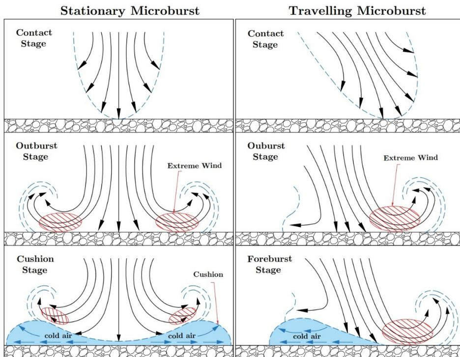
**Figure 4.** Schematic vertical cross-sections displaying the time evolution of the atmospheric flow across a stationary downburst (left column), and a typical moving or non-stationary downburst (right column) (based on Fujita [17]).
