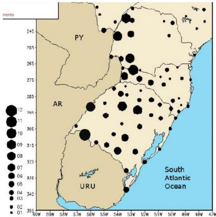
**Figure 9.** Climatology of wind gusts generated by severe storms in southern Brazil, based on measurements from the national network of INMET automated surface weather stations between 2005 and 2015. Diameters of the black circles are proportional to the number of occurrences of convectively-induced wind gusts equal to or greater than 25 m/s; see convention in ref. [29].
