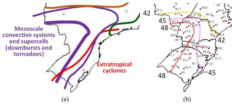
Figure 19. South region: a) climatic regions; b) proposed isopleths ( $V_0$  in m/s).
