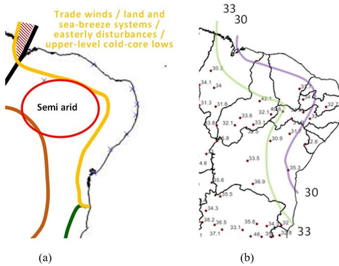
Figure 20. Northeast region: a) climatic regions; b) proposed isopleths ( $V_0$  in m/s).
