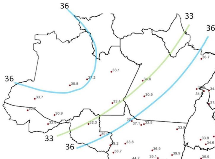
Figure 18. Amazon climate region and proposed isopleths,  $V_0$  in m/s.
