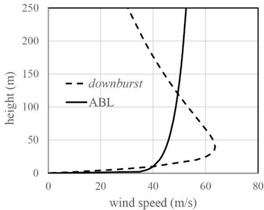
**Figure 3.** Mean wind profile corresponding to  $V_0$  equal to 40 m/s for atmospheric boundary layer winds (full line) and downburst-like winds (dashed line, with maximum at height of 40 m) during its horizontal divergence at low-levels, based on Vicroy model [20].
