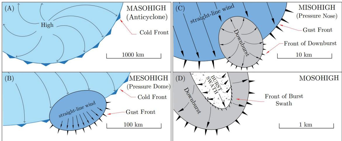
**Figure 5.** Schematic charts for the Northern Hemisphere displaying close up views of horizontal flow patterns originating from the combination of synoptic and non-synoptic winds forced by atmospheric processes belonging to different scales of motion. From (a) to (d), panels depict flow patterns at ever shorter horizontal scales (based on [17]).
