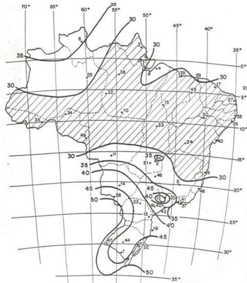
**Figure 1.** Isopleths map of current NBR 6123 [1].  $V_0$  values in m/s shown at tips of isocurves; numbers associated to dots identify the weather stations.
