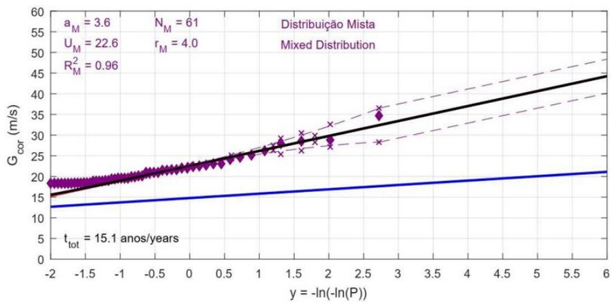
Figure 14. Distribution fit and data for maximum annual wind speeds at station SBBE in Belém, PA [7].
