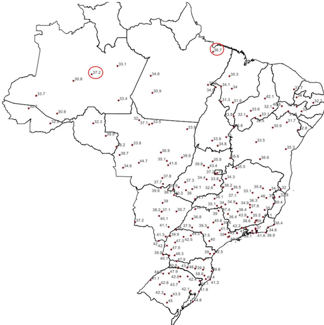
Figure 17. Overview of selected weather stations and corresponding  $V_0$  values (m/s) processed by Vallis [7].
