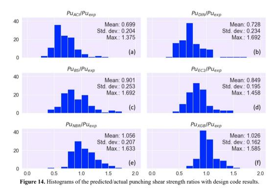
From Figure 14, the ACI, DIN, BS, EC2 and NBR models estimate, on average, failure loads 30.1% lower, 27.2% lower, 9.9% lower, 15.1% lower and 5,6% higher than the real ones, respectively. On the other hand, the XGB estimates values, on average, 2.6% higher than the experimental ones.
