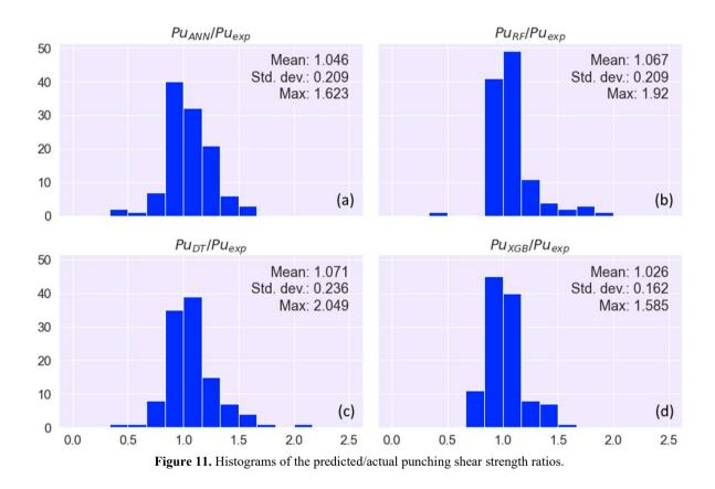
In applications related to structural engineering, it is essential to understand whether the model usually leads to values in favor of safety, that is, conservative, or not. In this sense, the method proposed in [48] is employed herein to compare the different ML models. Table 3 presents the calculated conservatism indexes (C) and indicates that all models are considered slightly non-conservative according to the method, with negative values.
