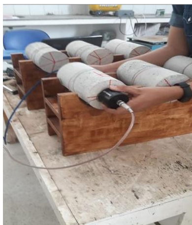
Figure 3. Specimens during measurement of ultrasonic pulse velocity.
