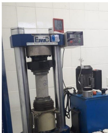
Figure 2. Specimen during compression rupture test.
