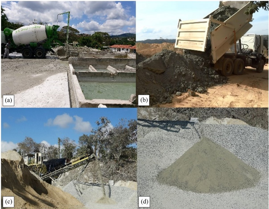
Figure 2. Stages of obtaining and processing the recycled aggregate. (a) Settling tanks; (b) Material discharge area; (c) Crushing; (d) recycled fine aggregate.
