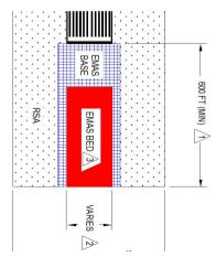
Figure 1. RESA and EMAS general arrangement at runway head (Source: Federal Aviation Administration [9])
