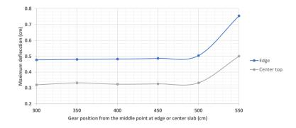
**Figure 8.** Maximum deflections caused by main gear A 320-200 on concrete.
