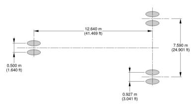
Figure 5. Distances between wheels and gears of A320-200 [28]
