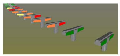
Figure 6. Variation of chloride levels in the crossbeams (Navisworks)
