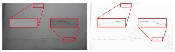
Figure 4. Surface without fissure (left) and surface with fissure (right)
