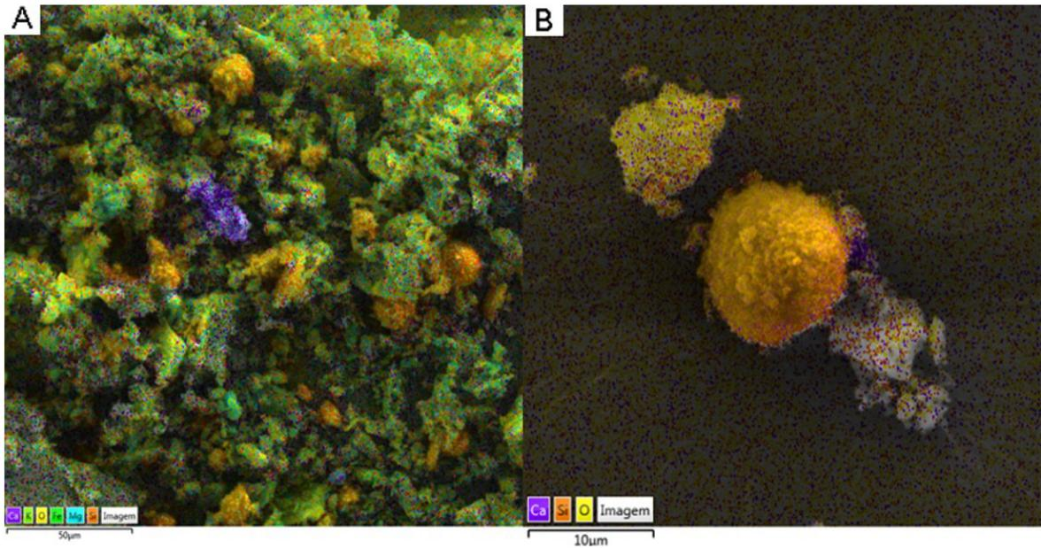
Figure 2. SEM of the murumuru husk ash at two distinct points (A) and (B) by EDS.
