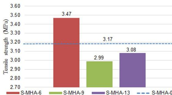
**Figure 5.** Result of the test for tensile strength by diametrical compression.
