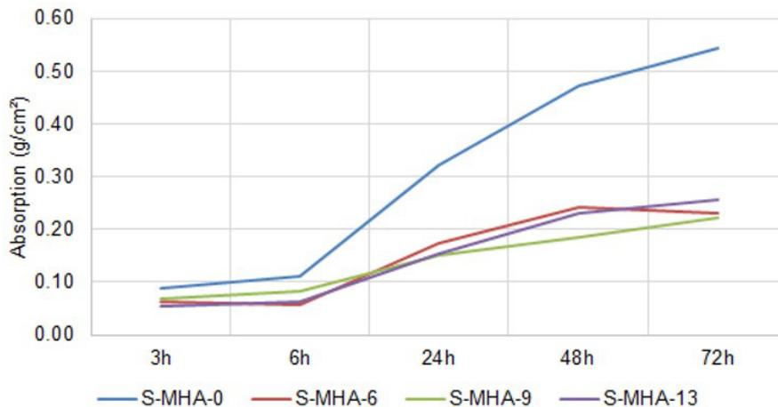
Figure 7. Water absorption by capillary suction (g/cm²).
