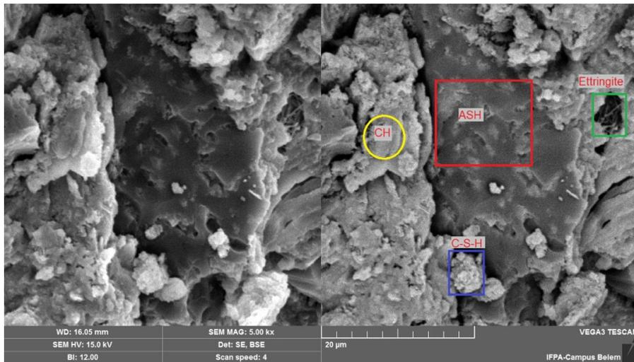
Figure 10. SEM of S-MHA-6 in a different region at 5k X
