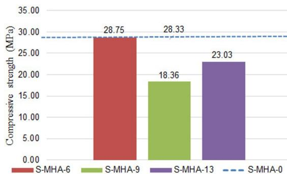
**Figure 4.** Result of the compressive strength test at 28 days.
