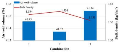
Figure 5. Bulk density and void content of the combinations
