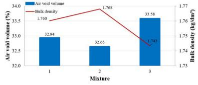
Figure 7. Bulk density and void content of mixtures
