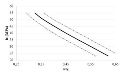
Figure 2. Relation between the w/c ratio and the average compressive strength, at 28 days
