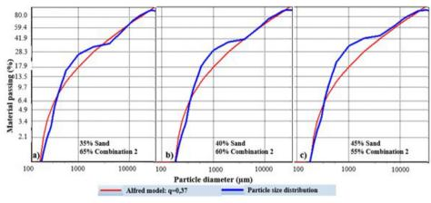
Figure 6. Gravel and sand grading curves by EMMA
