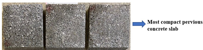
(c) Slabs with fine and coarse slag.
