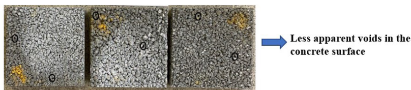
(b) Slabs with fine slag and 9.5 mm gravel.
