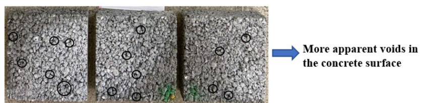
(a) Slabs with fine slag and 12.5 mm gravel.
