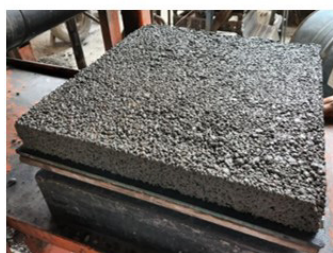
(c) Initial concrete slabs (50 cm×50 cm×6 cm).
