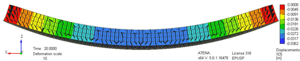
Figure 19. Displacement results and crack pattern - ISO834 time-temperature curve
