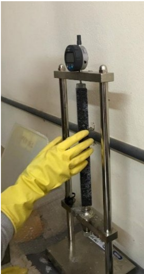
Figure 4. Measuring the dimensional variation of the specimens.
