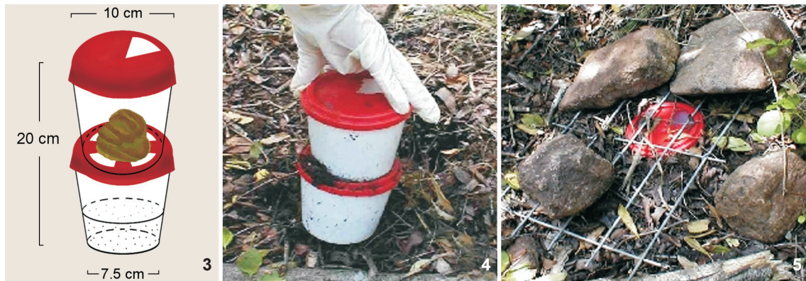
Figures 3-5. Schematic representation of the dung (or carrion) baited pitfall trap (3) used in this study containing the bait (above) and the fixative (below). The pitfall trap (4) before being buried with the rim at ground level (5).
