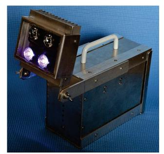
Figure 1. View of the device with the movable head upright and UV LEDs on. Scale: 10 cm.
